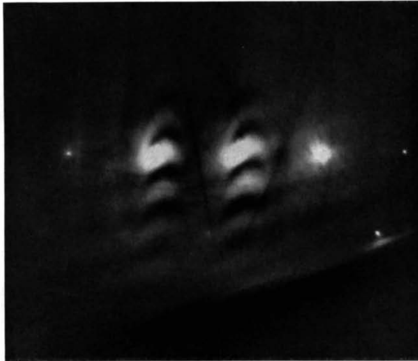
Fig. 5. Diffraction pattern of silicon obtained under conditions such those shown in Fig. 1(b), at 80 kV. The Bragg condition is not exactly satisfied for the 111 reflexion. Two kinds of contrast effect are observed, as illustrated in Fig. 6(a).
